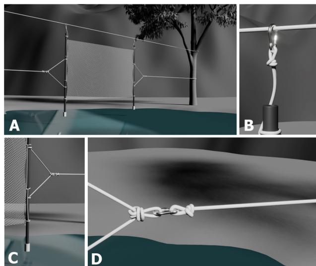
Fig. 1 - The skynet design. A. Overview of the skynet *in-situ* (over-water). B. Attachment to tension line. C. Attachment of poles to lateral lines. D. Knotwork of lateral lines.
